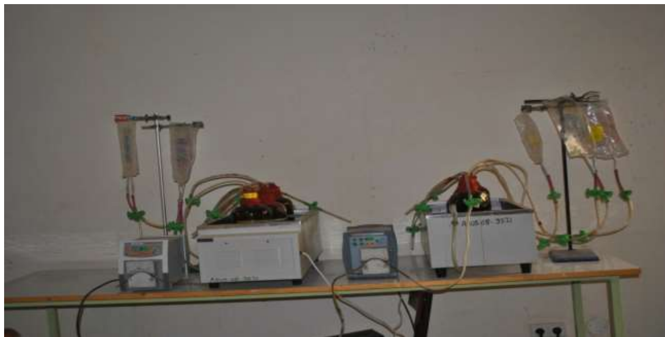
Figure 1. The two-stage ASBR setup.
